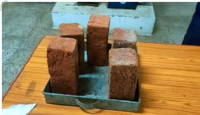
Figure 10: Efflorescence is observed after 7 days
