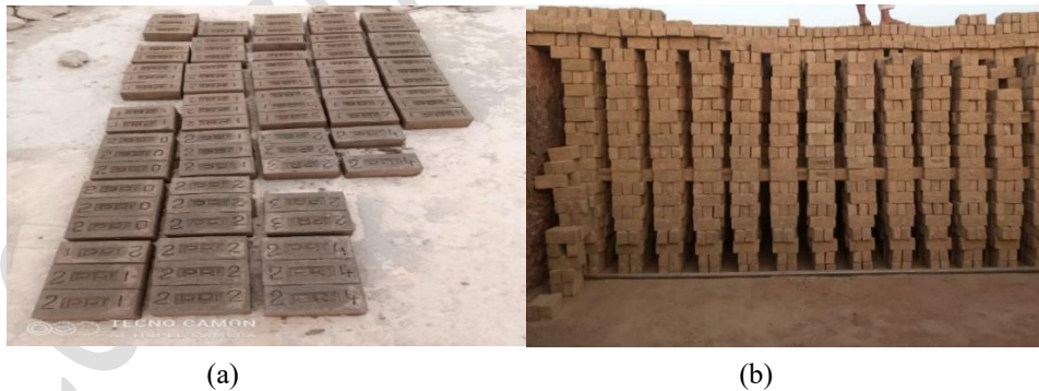
Figure 3. (a) Bricks placed for drying, (b) Arrangement of bricks for kiln firing.
