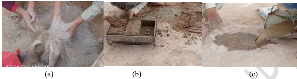
Figure 2. (a) Soil mixing with other ingredients, (b) Hydration Process, (c) Moldings Process.
