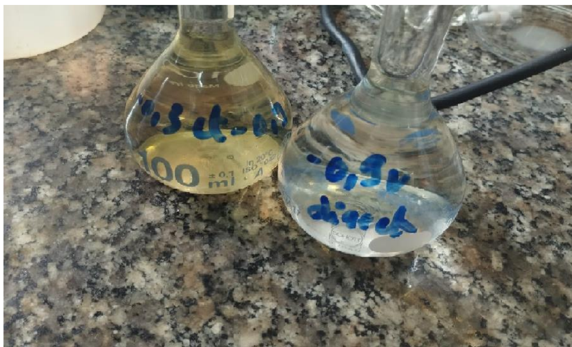
Figure 13. Nessler's reagent test of the electrolyzed solution after successive electrolysis at -0.4 and -0.9 V vs. SCE, confirming the presence of ammonium ions.
