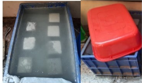
Figure 4. Cube specimens placed in alkaline medium
