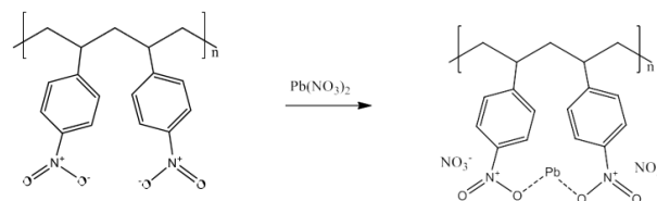
Figure 12. The interaction of Pb^{2+} with NO_2 anionic group from the adsorbent
